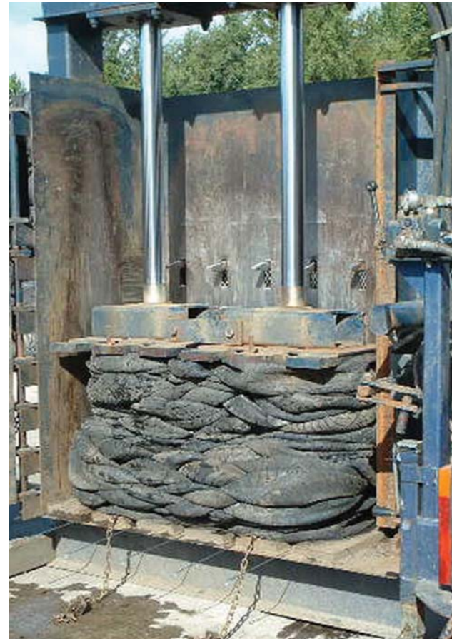
Figure 4 – Tyres compressed in a typical baler prior to locking into position to allow the addition of further tyres
