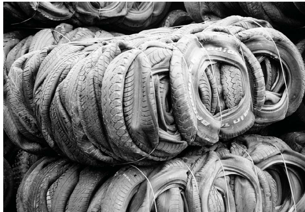
Figure 13 – Completed tyre bales
