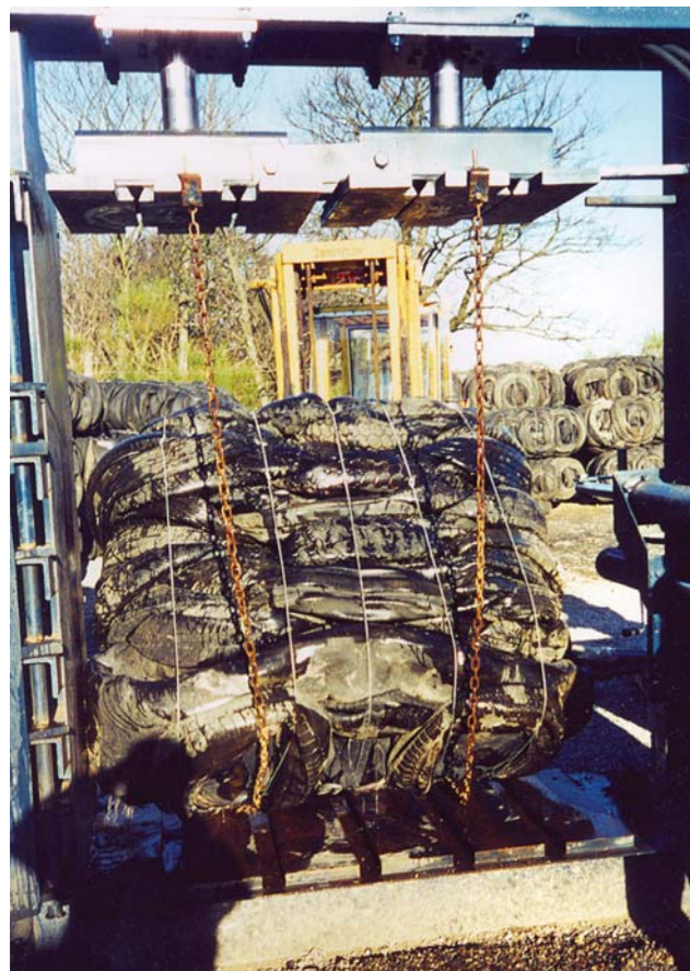
Figure 11 – The chains tip the bale out of a typical baler
