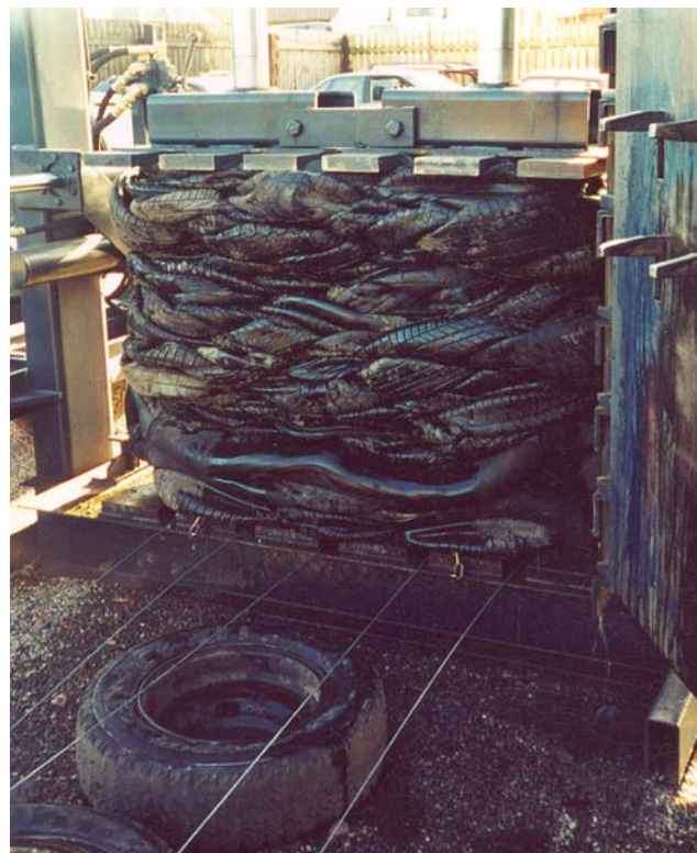
Figure 7 – A fully compressed bale with tie wires ready to wrap around a bale manufactured in a typical tyre baler
