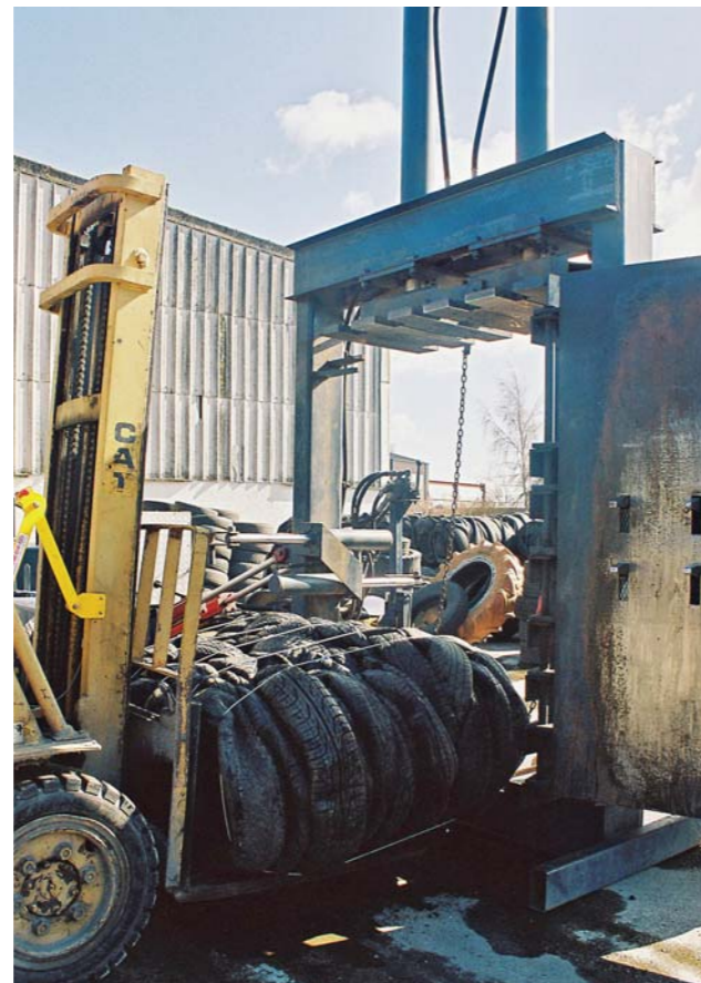
Figure 12 – The bale is removed from a typical baling machine
