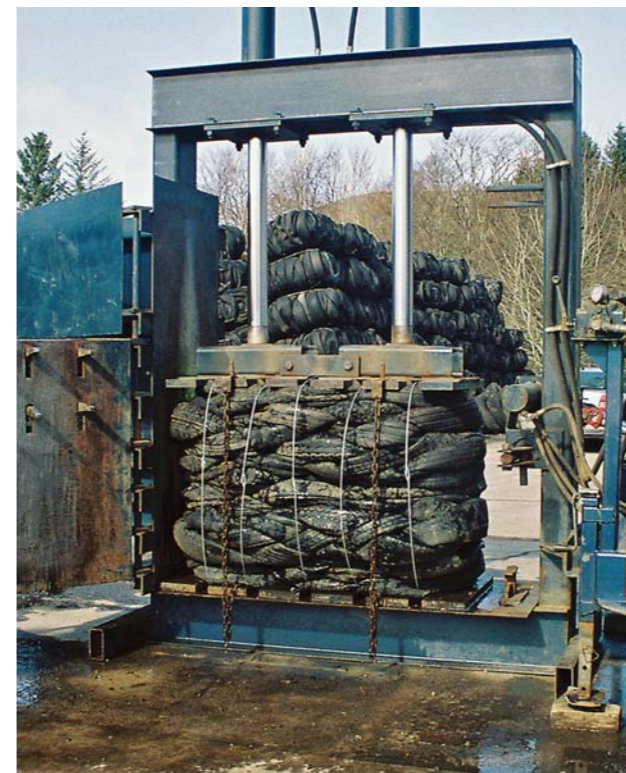
Figure 9 – A typical fully compressed bale with tie wires in position and the bale removal chains secured to the front of the top platen
