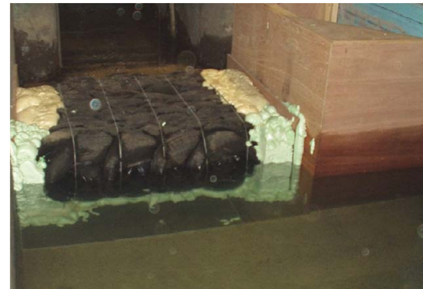
Figure C.1 – Bale in flume for permeability testing showing (timber) flume inserts and foaming sealant between bale and flume/insert walls
