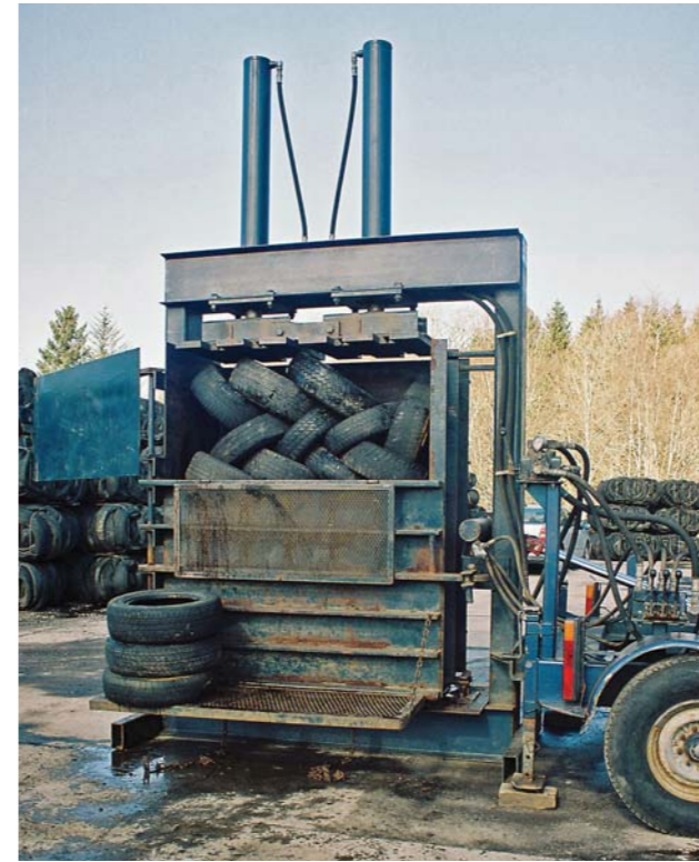
Figure 5 – Further tyres added to the bale ready for further compression. A typical tyre baler is shown
